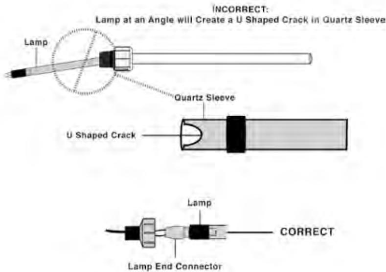
**Lamp Dropped into the Quartz Sleeve can cause Breakage**
